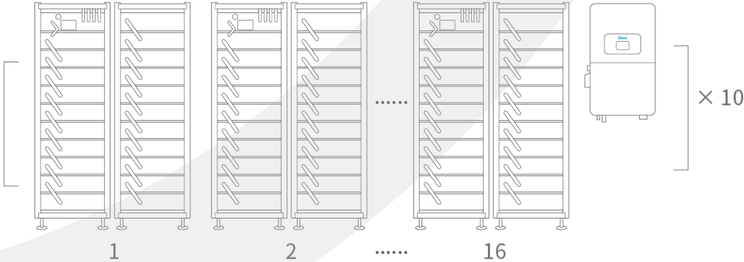
Maximum support for 10 inverters in AC parallel operation
