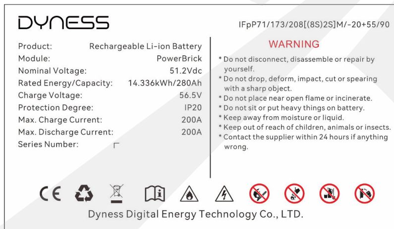
Figure 1-1 Battery Energy Storage System nameplate
